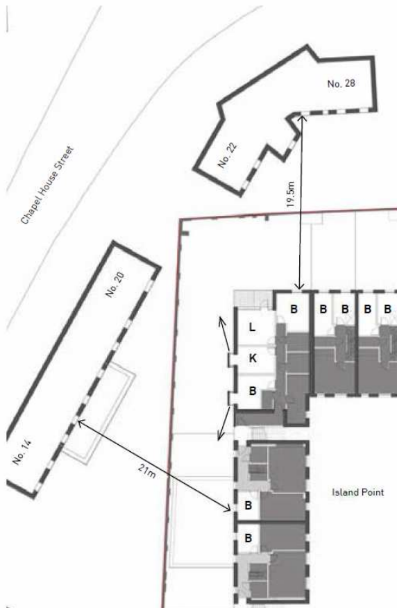
Overlooking study - north west corner, first floor
